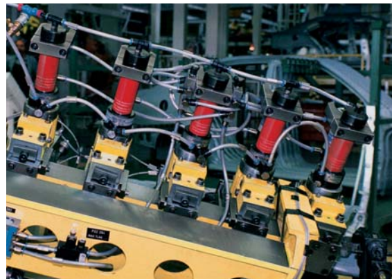
Stamping units placed in line
