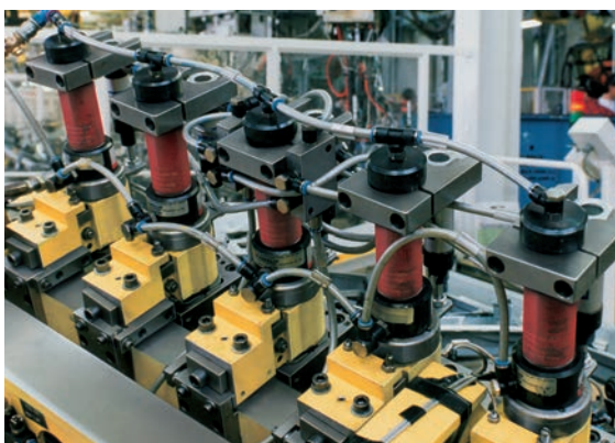
Stamping units placed in line
