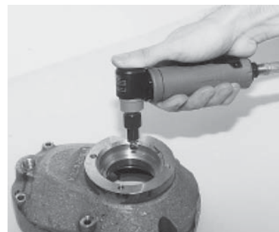
Deburring with an ball shape bur and a 12S1200-36
